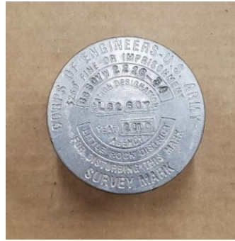
Figure 2: Aluminum Survey Marker
