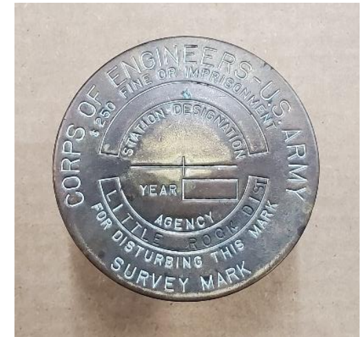
Figure 1: Brass Survey Marker
